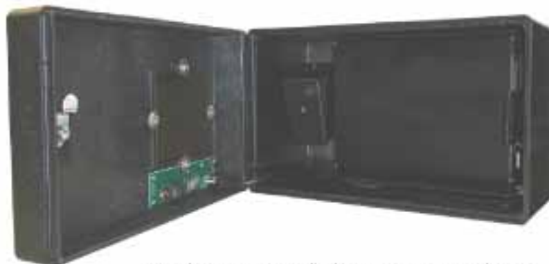
Digital 7200 DVR installed into a BC 2000 Enclosure
