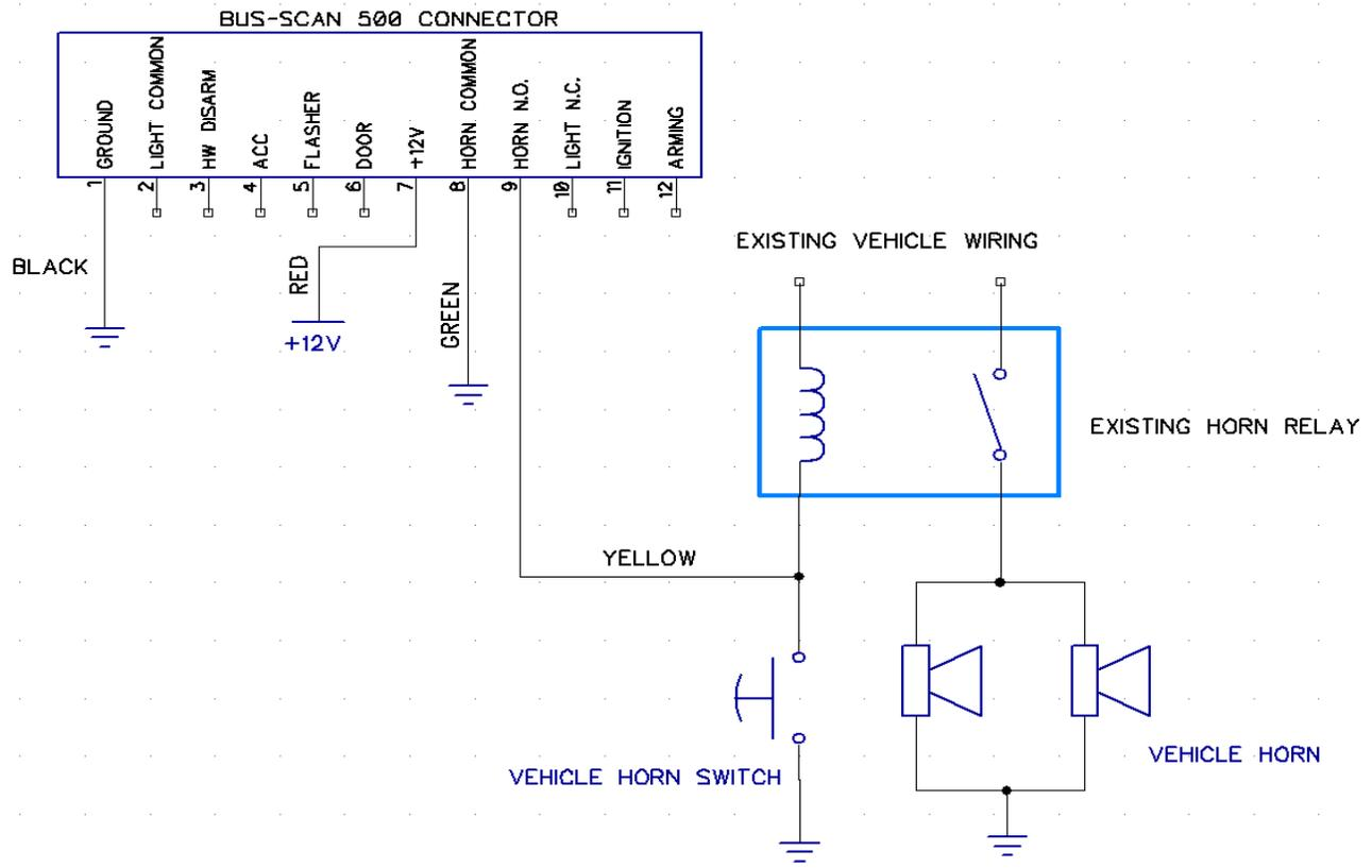
**IMPORTANT:** Never connect the Bus-Scan 500 Horn Relay output directly to the vehicle horn. Always connect to the COIL side of the existing vehicle horn relay. Failure to observe this practice can create a hazard and damage the Bus-Scan 500 system (as well as void the warranty)
